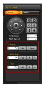
Setting and recalling Presets can easily be programmed using the control section of the PTZ controls. You can recall Tours here but programming of Tours is carried out in the camera menu itself going through the menu or by pressing the Tour shortcut button.
