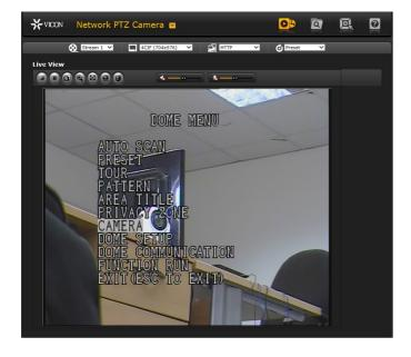
The Dome menu is accessed using the PTZ and lens controls to increment settings and/or to enter/exit settings.
