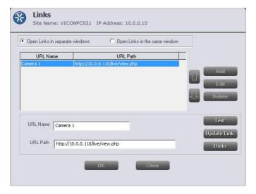
To facilitate any camera programming you can preprogram the camera IP addresses into the Links section of ViconNet. This will give you give quick access to the web browser.
